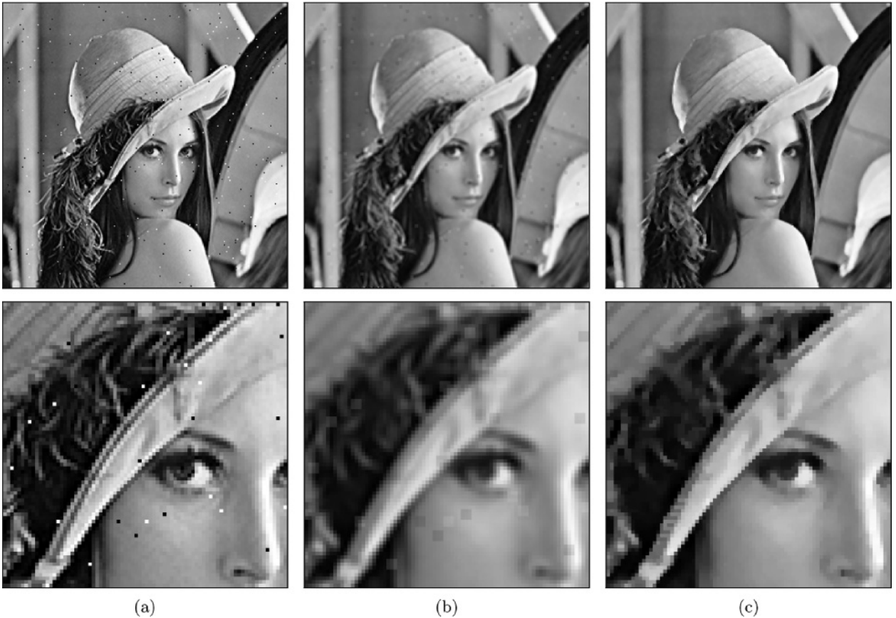
Fig. 6.18. Linear smoothing filter vs. median filter. The original image is corrupted with “salt-and-pepper” noise (a). The linear 3 \times 3 pixel box filter (b) reduces the bright and dark peaks to some extent but is unable to remove them completely. In addition, the entire image is blurred. The median filter (c) effectively eliminates the noise dots and also keeps the remaining structures largely intact. However, it also creates small spots of flat intensity that noticeably affect the sharpness.
