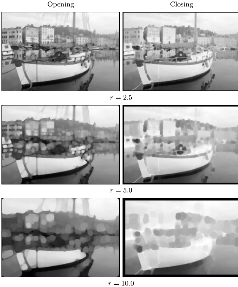
Fig. 10.23 Grayscale opening and closing with disk-shaped structuring elements. The radius r of the structuring element is 2.5 (top), 5.0 (center), or 10.0 (bottom).
